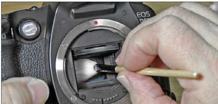
Allen Skoreyko cleans the sensor on his Canon EOS D60 using the Sensor Brush™ made locally in Edmonton.
